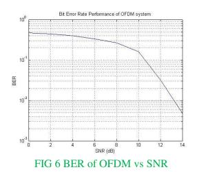
The following simulation result showing BER performance of Turbo Coded OFDM
