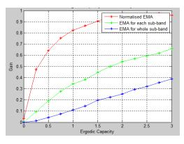
Figure 3: Comparison of gains of different MA methods for M = T = 30, N = 40, and U = 700.
