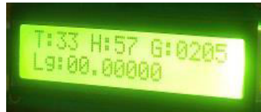
FIGURE 4:After detection of the temperature, humidity, gas, location at coal mine
