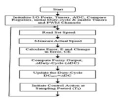
Fig. 6. Flowchart of a fuzzy controller program.
