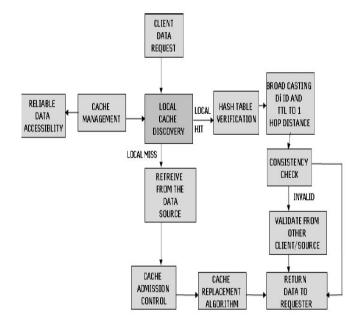
Figure 3 – Illustrates hybrid approach for cache invalidation [3]
