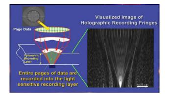
Illustration of what the holographic image looks like as it is being written onto the recording layer.
