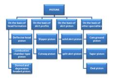
Fig 1.1: Hierarchal representation of piston types
