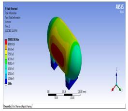
Figure 5.1 shows the Total deformation of the pressure vessel formed with stainless steel material
