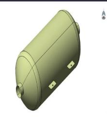
Fig 3.1 Cylindrical pressure vessel Model
