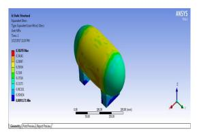
Figure 5.2 shows the equivalent stress analysis on pressure vessel of stain less steel material
