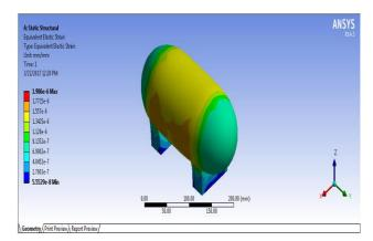
Figure 5.4 shows the Equivalent Elastic strain of pressure vessel of stainlessteel material
