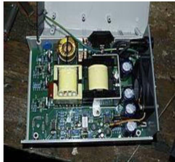
Fig2. Inside of a SWEA 250W Transformer-based grid-tie inverter.
