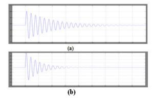
Night time (a) generator power Pg (B) infinite bus power Pinf
