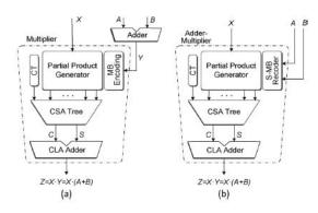
Fig. 1. AM operator based on the (a) conventional design and (b) fused design with direct recoding of the sum of A and B in its MB representation.
