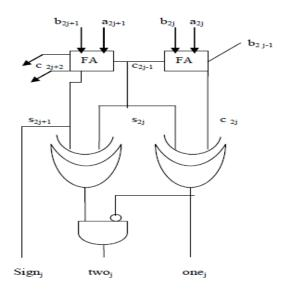
Fig. 3Circuit diagram for proposed MBRS
