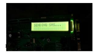
**Car Theft Identification:** A system operation is triggered when a limit switch is tripped . When the limit switch is pressed, theft alert is displayed on the LCD screen and SMS along with location of toy car is given to the number that is pre fed via GSM Modem. In real life SMS would be sent to the owner of the vehicle along with the location of the car, as in Fig.6.3
