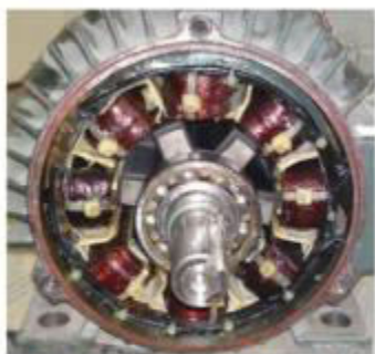
Figure 1. The tested 8/6 SRM inside view.
