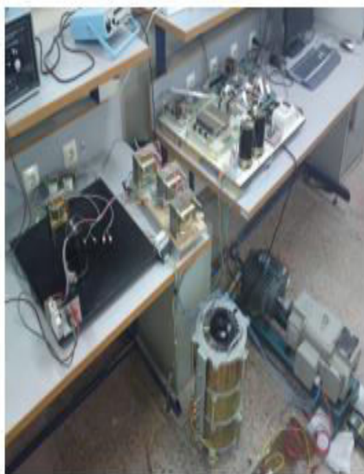
Figure 7. SRM drive test setup used for experimentation.
