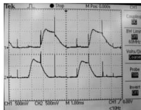
Figure 8. phase current of SRM (scale: phase current= 1.75A/div).
