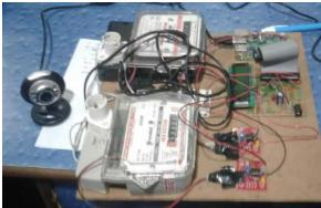
The Raspberry Pi 3 provides a supply of 5 V but the electrical appliances in general operates on 230 V. So relays are employed in this system for voltage conversions and also to remotely ON and OFF the electrical appliance. The energy consumed by the two
