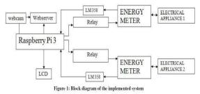
**Relay:** Relay shown in Figure 3 are used to split and set up connection so as to pass the current. Its significant application is to act like a switch. Relays are used in controlling and monitoring applications. The electrical appliances operate on 230 V, but the Raspberry Pi 3 works on 5 V. So to overcome this problem relays are used.
