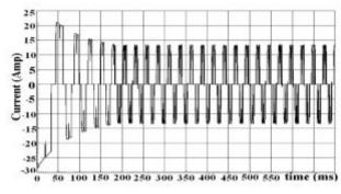
Fig 8. Simulation result for phase current response of BLDC motor on full load (1151 rpm)
