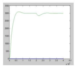
x-axis :- Time (sec) y-axis :- Speed (RPM) Fig 4 Speed Characteristics of bldc
