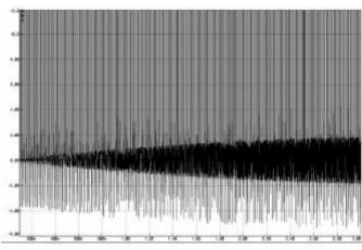
Fig.7 BLDC motor voltage waveform equivalent to 1500 rpm speed
