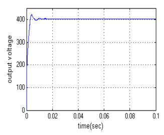
Fig.12.output Voltage of high step up Converter.
