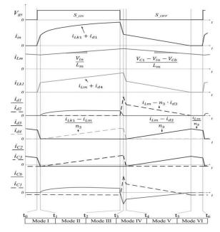
Fig. 3. Steady-state waveforms in CCM operation.
