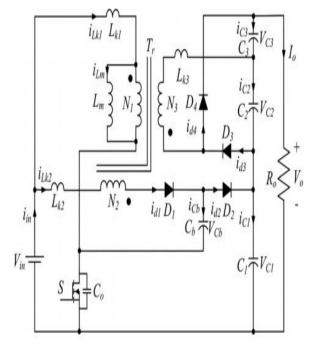
Fig. 2. Equivalent circuit of the proposed converter.
