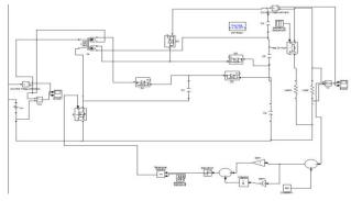
Fig.19.Matlab/simulation model of Closed loop Control of high step up Converter with Decremental load.
