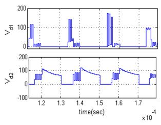
Fig.10.Simulation waveform of diode Voltage (Vd1), diode Voltage (Vd2).
