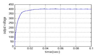
Fig.14.output Voltage of high step up Converter with fuel cell.
