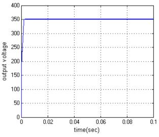
Fig.16.Output Voltage of high step up Converter with closed loop Controller.
