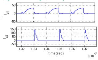
Fig.8.Simulation waveform of diode Current (Id1), diode Current (Id2).
