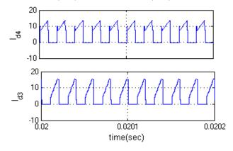
Fig.9.Simulation waveform of diode Current (Id4), diode Current (Id3).
