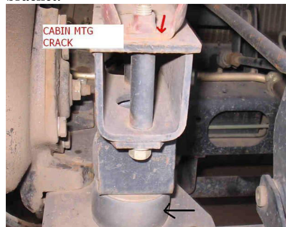
Fig:1.1 show the practical problem of the mounting bracket. The red mark shows the mounting bracket failure
