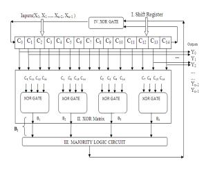
Figure 2: existed plain ML decoder
