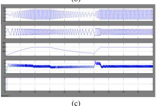
Fig.7 Dynamic performances of the proposed SPV array-based zeta converter-fed BLDC motor drive for water pump. (a) SPV array variables. (b) Zeta converter variables. (c) BLDC motor-pump variables.
