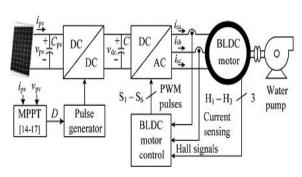
Fig.1. Conventional SPV-fed BLDC motordriven water pumping system
