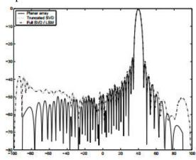
Figure 3: Destination pattern and synthesized patterns obtained with the least-squares solution and the leastsquares approximate solution for a scan 40° away from broadside
