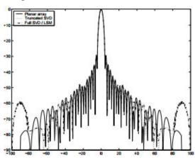
Figure 2: Destination pattern and synthesized patterns obtained with the least-squares solution and the leastsquares approximate solution for a broadside scan
