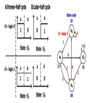
FSM of FM0 uppose the initial state is S1, and its state code is 11 for A and B, respectively.
