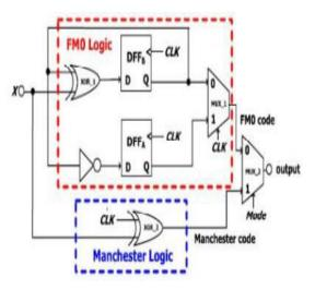
This is the hardware architecture of the fm0/Manchester code. the top part is denoted the fm0 code and then the bottom part is denoted as the Manchester code. in fm0 code the DFFA and DFFB are used to store the state code of the fm0 code and also mux\_1 and not gate is used in the fm0 code. When the mode=0 is for the fm0 code, the Manchester code is developed only using the XOR gate and when the mode=1 is for the Manchester code.
