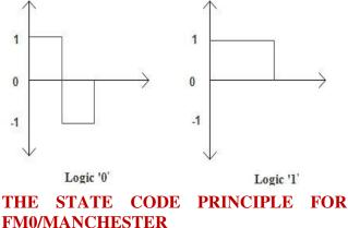
The Manchester encoding is an XOR operation only. The FM0 code starts with the FSM principle. The FSM of FM0 code classified into
