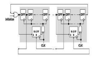
The above block diagram shows the power controlled Ring counter.First, total block is devided into two blocks. Each block is having one SR FLIPFLOP controller
