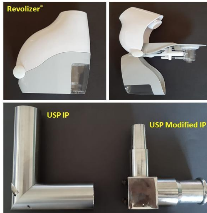
Figure 1 Revolizer inhaler device and US Pharmacopoeia (USP) induction ports (IP) i.e. USP IP and USP modified IP.
