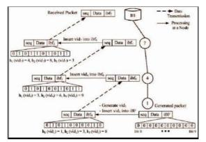
Figure1: Mechanism for encoding provenance (node 1 is data source).
