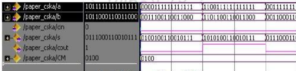
Figure 7: Waveform of Proposed-CSKA
