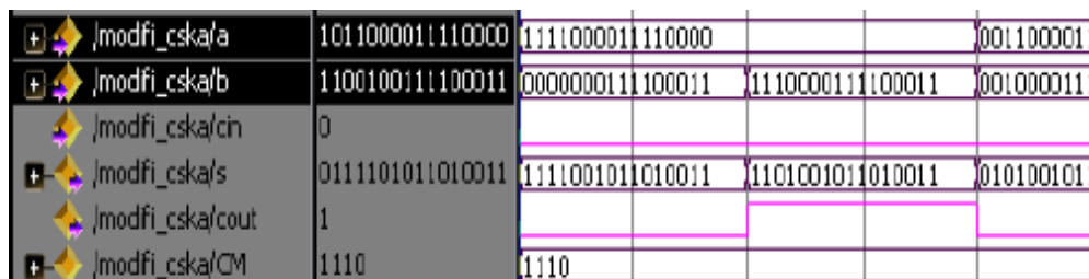
Figure 8: Waveform of Modified-CSKA
