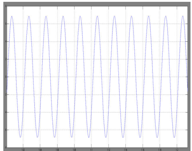
Fig.21 Output waveform of Rectifier Input Current i_{g1}
