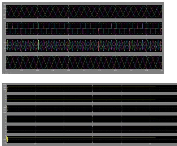
Fig.8: Simulated performance of the proposed DFIG-based WECS working as a STATCOM at zero wind speed.
