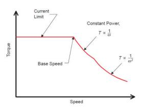
Fig.3 SRM Torque-Speed Characteristics
