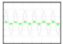
Fig.15 Simulated input wave form of Voltage and current for closed loop controlled SRM Drive
