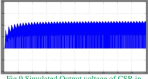
Fig.9 Simulated Output voltage of CSR in openloop SRM Drive
