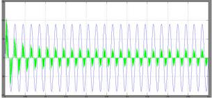
Fig.8 Simulated input voltage and current waveforms for SRM drive with CSR
