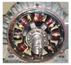
Fig.3 The tested 8/6 SRM inside view
