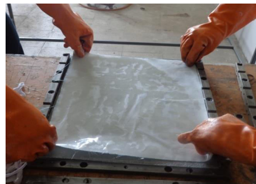
Placing first the ply
